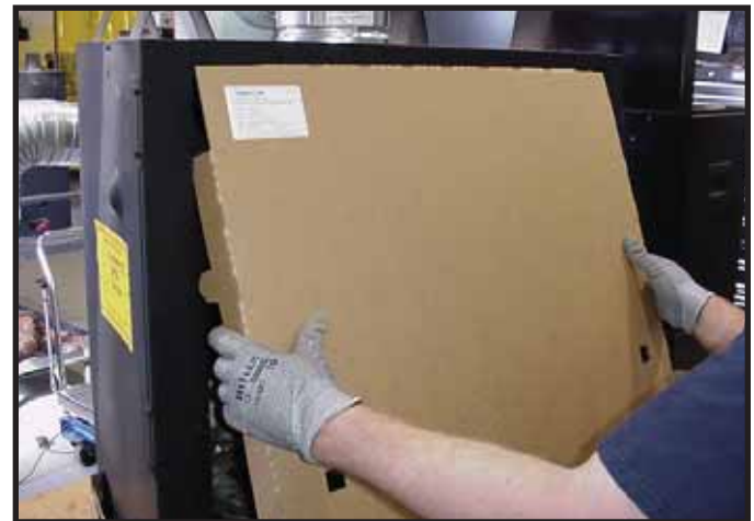
Figure 13.4 Installation of Splatter Guard
